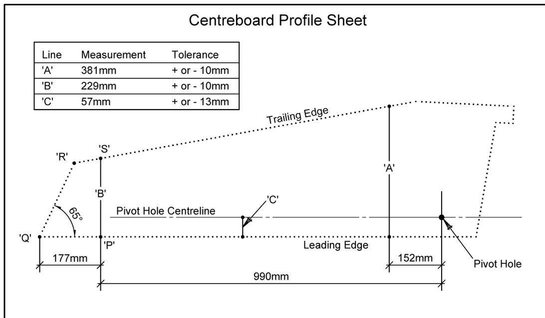
Measurements A, B and C are taken at 90° to the leading edge at the stated distance from the centre of the pivot hole. They shall be within the limits of measurement given on the Centreboard Profile Sheet.
