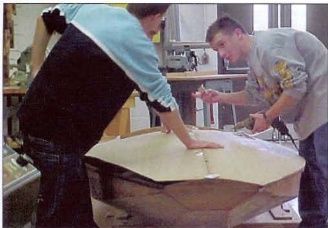
Students in David White's shop class build the wide-bow Fireball on a setup of male molds, which help the builders remain faithful to the hull's intended shape.
